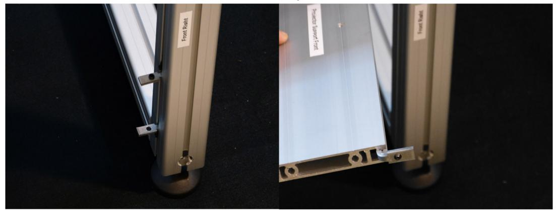
Slide the brackets into the slots on the feet of the machine. Note This image demonstrates how the Projector support should fit into that the SHORTER bolt should be facing the slot and the LONGER the brackets. Note the orientation of the bracket since you shall be bolt should be outside.
