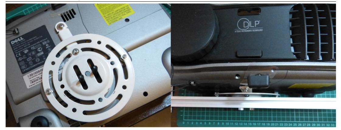
Note the Single Mount Arm and the screw positions. The bottom two screws should go through the pre-drilled holes on the mount. Don't forget to run through the two Allen Bolts on the back of the mount before screwing the mount to the projector. The Bolts should also have a Washer on them.
