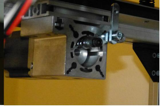
Install the VAT motor as shown in the image above. Once again, note the orientation of the wires.
