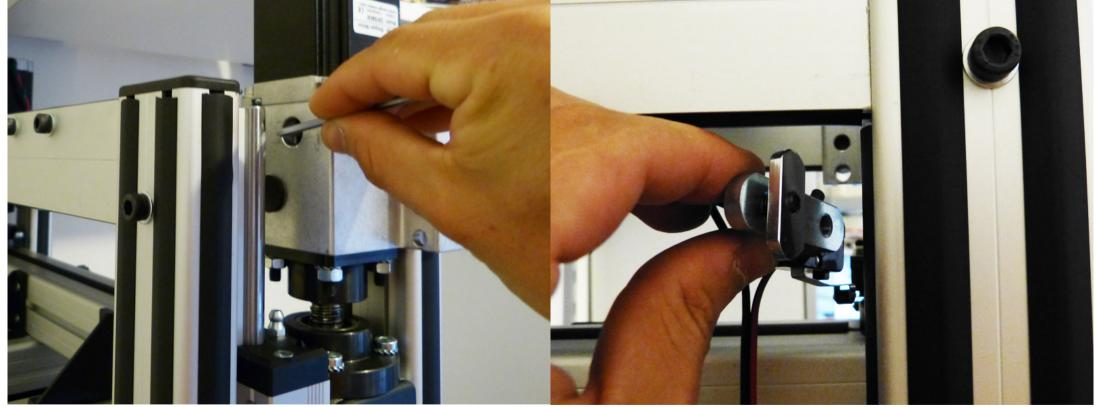
Tighten the Motor Coupling to the Motor Shaft through the openings in the Motor Mount. The orientation in which you installed we are installing the switch is the Left FRONT Motion Frame (the the Motor Coupling plays a great role in how easily you are able to image shows the Back view but it should be installed on the Front
