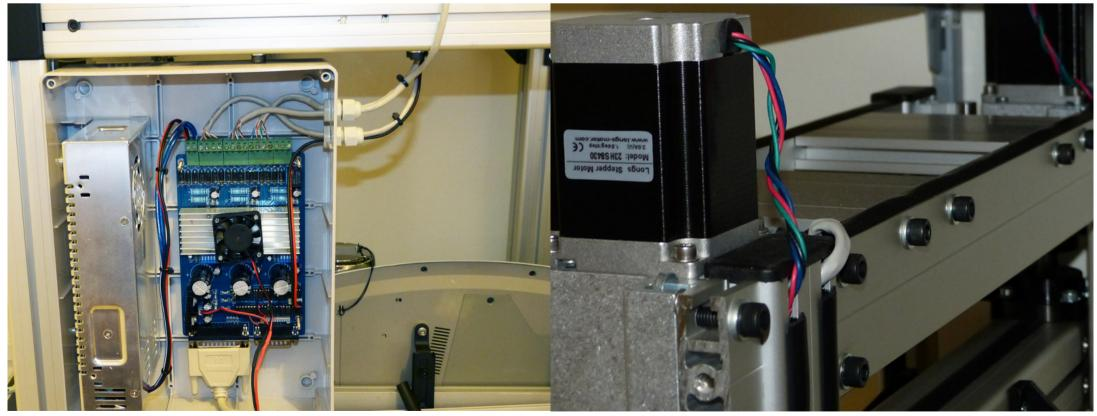
Install the Enclosure as shown in the image above. There are 2 6mm bolts already installed in the pre-drilled locations on the
