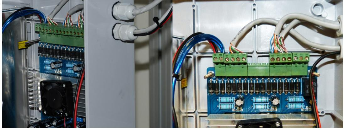
Guide the motor wires through the wire bushings as shown on the Connect each motor to the corresponding connector as shown. The image above. There should be plenty of space to fit them through. In which bushing you fit the wires is up to you, since there should motor. The other two motors should be connected to the Second or be enough cable length to connect them later on.
