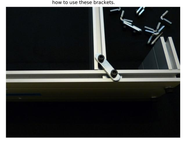
Mount the sub-assembly as shown to secure each projector mount to the frame.
