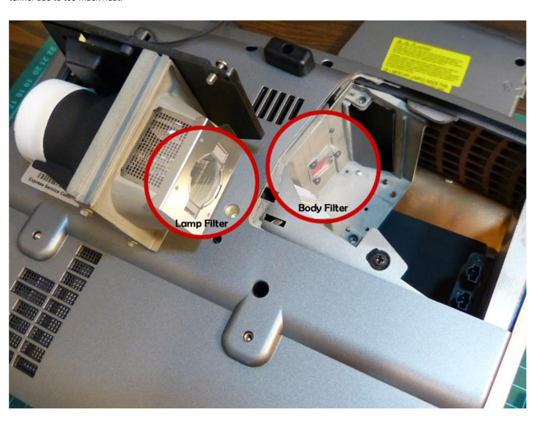
One of the filters shall be located in most cases within the lamp assembly itself, a second filter shall be located directly in front of it on the projector enclosure. You need to remove both filters to get the full light power.
