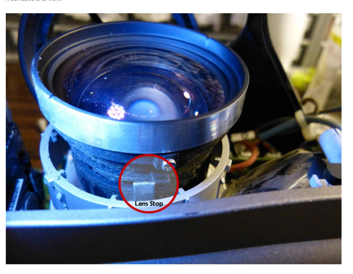
Almost all projectors have a stop mechanism which doesn't let the lens to be unscrewed or removed from the assembly. In most cases, disabling or removing this stopper shall give you the additional turns to focus. In some projectors this stopper is just a metallic piece which can be easily bent, in other cases it is a physical screw which needs to be removed.
