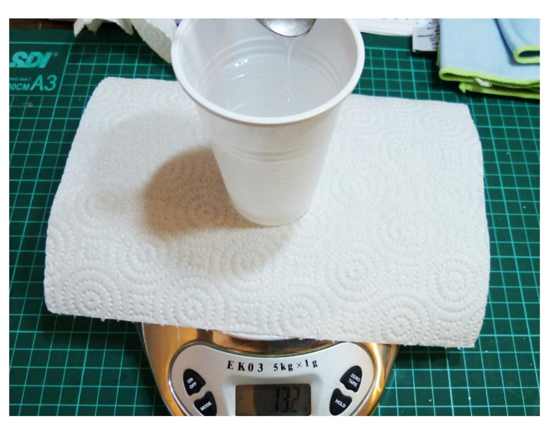
For this demonstration we use 132gr in TOTAL for the Small VAT. This comes to 120gr or PDMS and 12gr of hardener. Mix the two well for not less than 15 minutes before pouring into the VAT. The chemical reaction of the PDMS will take a long time to complete so you have at least 2 - 3 hours before it starts to settle. Do not worry about the air bubbles as they shall come out on their own later.
