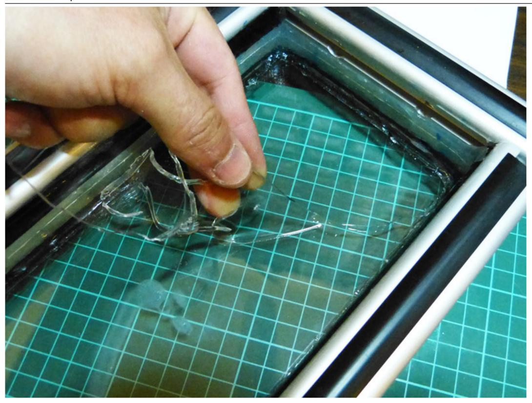
Continue peeling off the layer until none is left. Dispose of it and clean the glass surface well with a Micro-Fiber cloth and Acetone or Alcohol. If you pause before applying a new layer of PDMS, make sure to cover the glass so that no dust settles on top of it.
