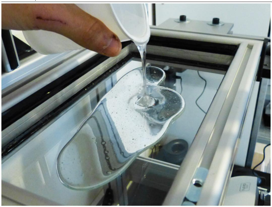
After stirring well the mixture, pour it on to the CLEAN surface of the VAT glass. Don't forget to clean it well with alcohol and try to avoid as much dust as you can. Start pouring from the middle and make your way to the edges. Do not worry about not covering the entire surface, it shall even out on its own after 30 minutes.
