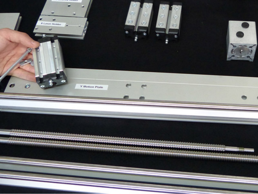
Since the slide blocks and the rail are pretty close to each other, we need to install the slide block and fasten it first, before we tighten the slide rail.
