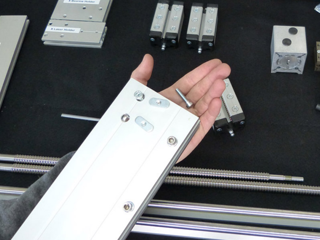
You shall notice here that we already installed the bolts for the motor support as well as the bolts for the slide block and its sliding nuts. Do it now as we shall be putting it all together later.
