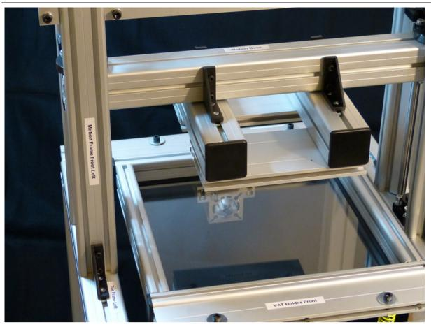
From the above image you can see the finished assembly. An additional option is to glue the Black glass onto the lift assembly with the included Epoxy. However it is recommended to first use the machine with the Aluminum surface since it tends to stick a bit better to the initial layers of the build.
