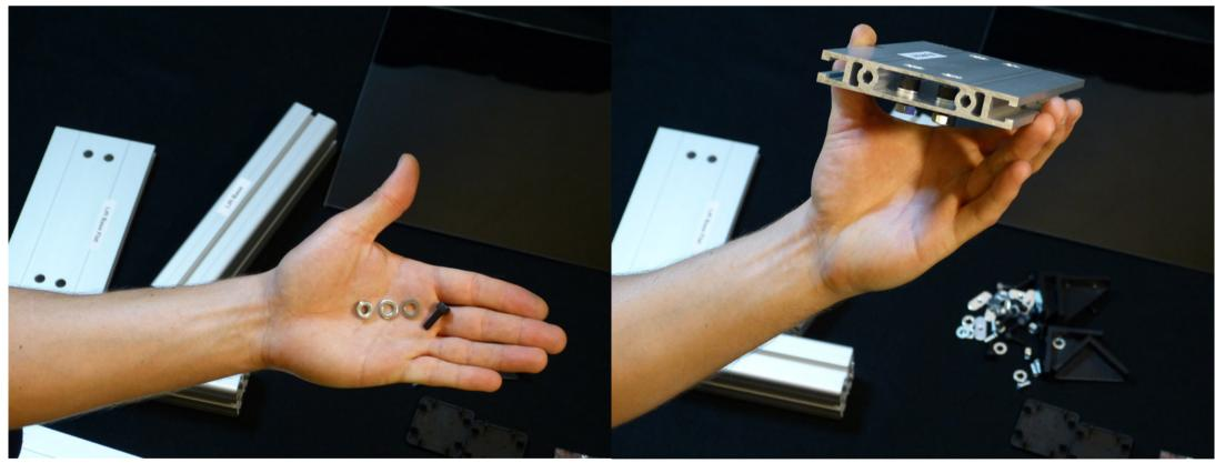
Get the 6mm Bolt, 2 washers and the 6mm nut from the Nuts and Position the 2 washers and the bolt as shown in the picture above.
