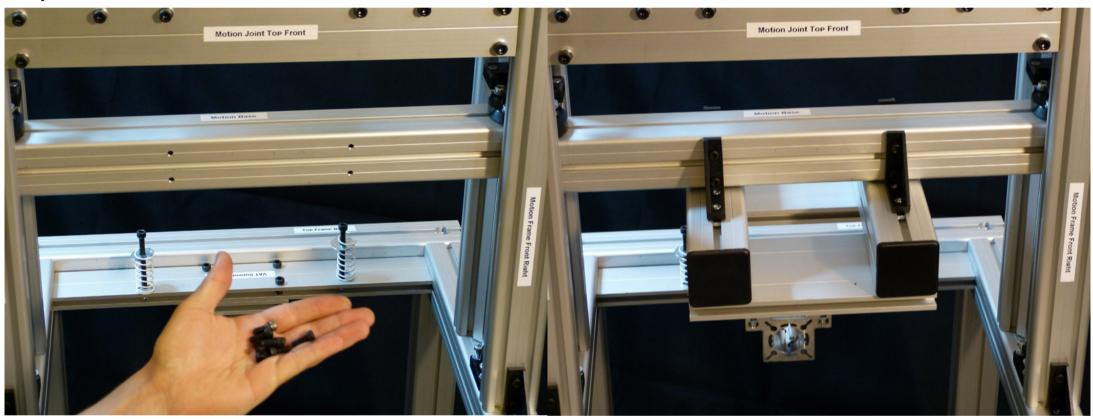
In the bag you shall find the 5mm bolts to secure the Lift on the Motion Base. Use them on the corner brackets as shown in the next assembly image. Secure the Lift Base onto the Motion Base as shown. Tighten the bolts all the way now and make sure everything is as level as possible.
