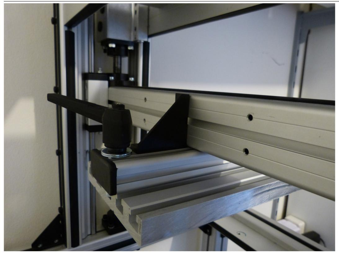
In the image above you can see how the Small Lift is mounted on the Lift Arm. The screw holes should already be on the arm so all you need to do is mount the lift as shown. If you purchased Both Large and Small lifts then use the bolts provided from ether assembly.
