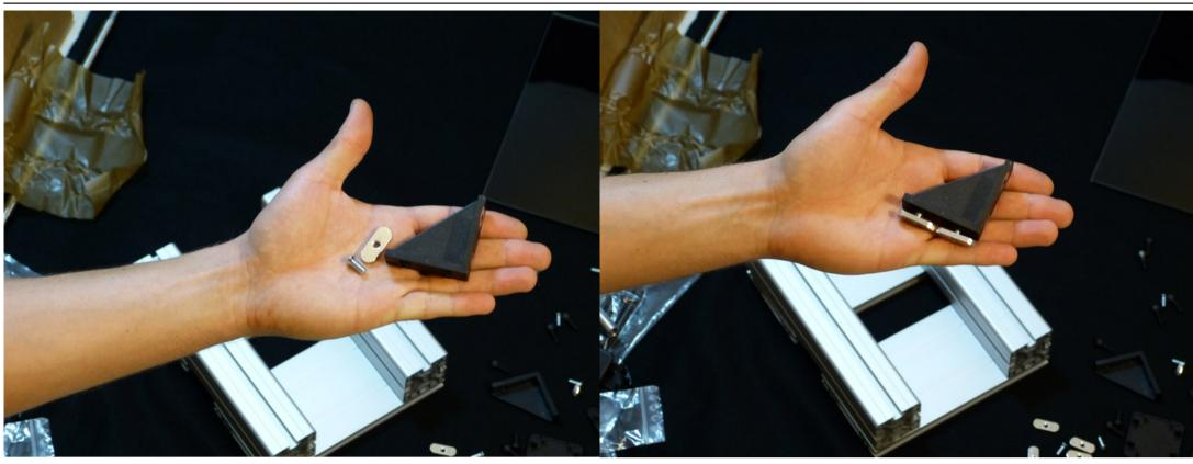
Get the corner brackets and the corresponding 5mm bolt and OvalAttach the bolts and nuts as shown on the picture. Make sure NOTSliding nut.to tighten them for now, since this shall have to slide into the
