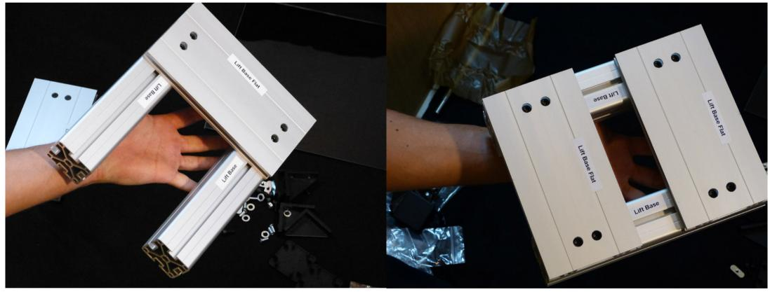
Do the same for the other Lift Base but don't tighten everything all the way just yet. Add the second Lift base flat as shown on the picture, tightening the bolts all the way now so that the assembly remains straight.
