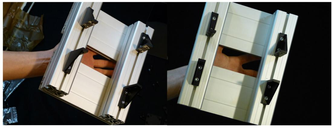
Slide the brackets as shown and make sure the walls of the corner brackets are facing outwards (esthetic reasons)
