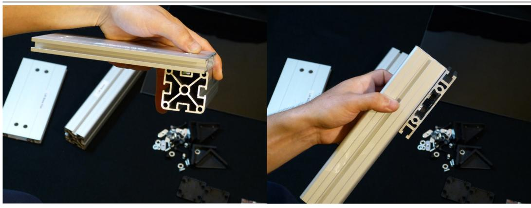
Take the Lift Base and slide it through the nut as shown on the image. Tighten it slightly to stay in place for now.
