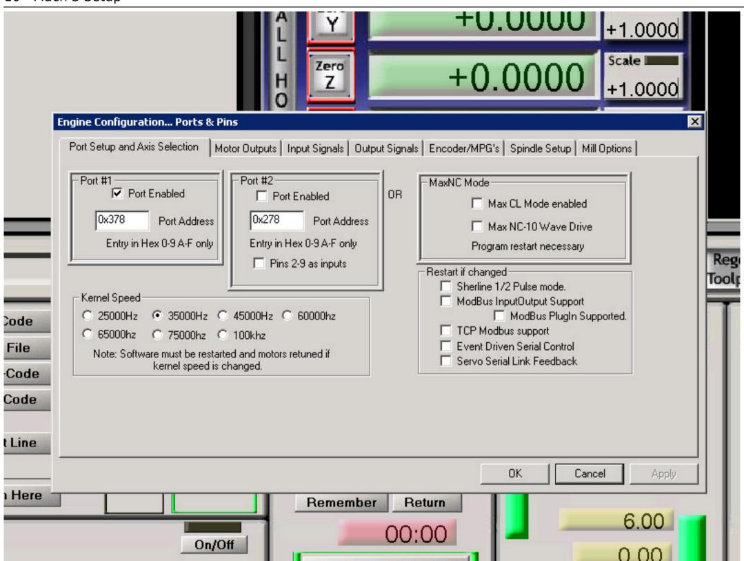
Note how the settings are setup in the Port Setup tab. Configure your tab to look just like shown on the image. The most important configuration to note is the Kernel Speed, which should be set to 35000Hz.
