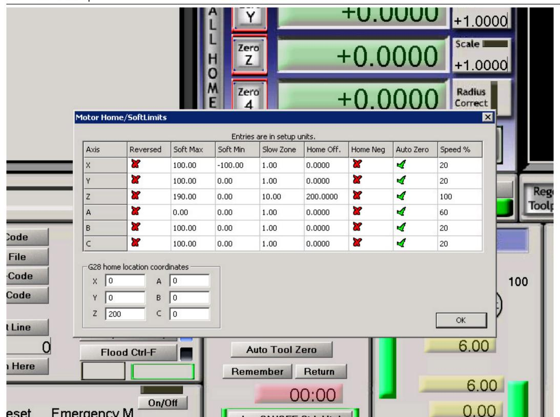
Set the numbers and other settings as shown on the screen. Don't forget the Reversed, home Neg and Auto Zero checks. Note that the number 200 is the Absolute Maximum position to which the Lift can go. To check this you can do the following:
