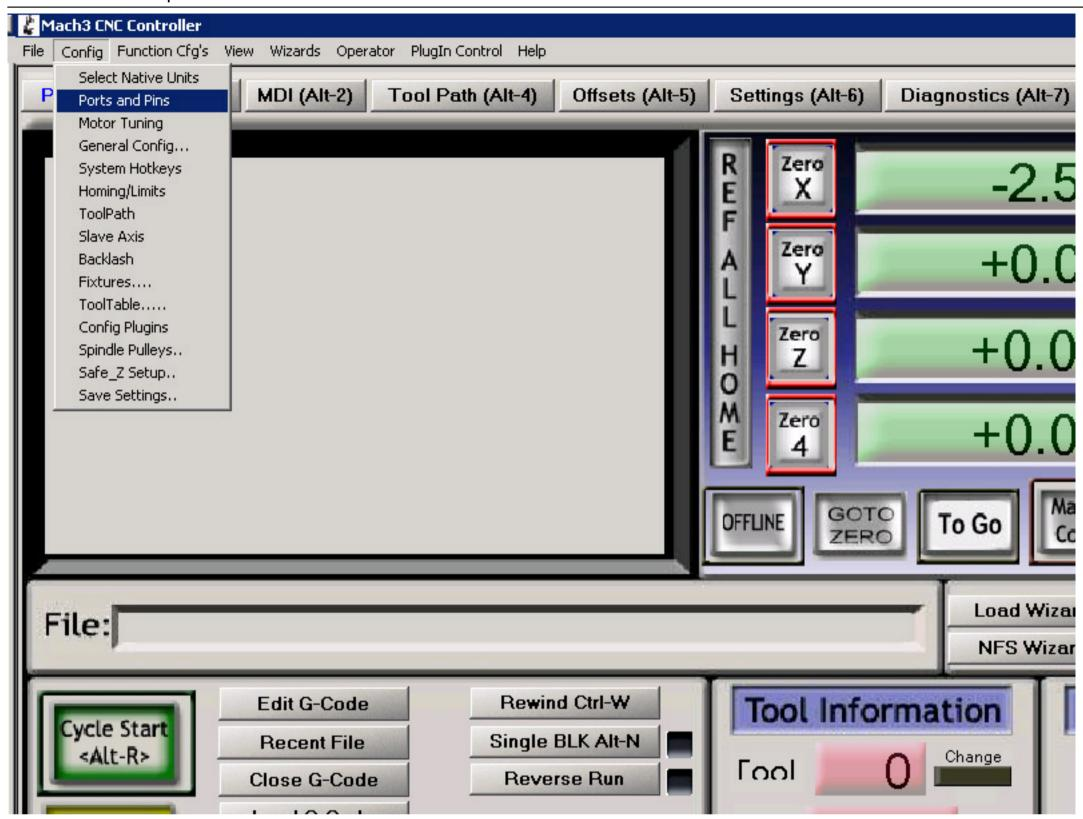
Next we need to setup the signals for the machine, so that Mach knows what to control and how. Use the Ports and Pins tab to configure this step.
