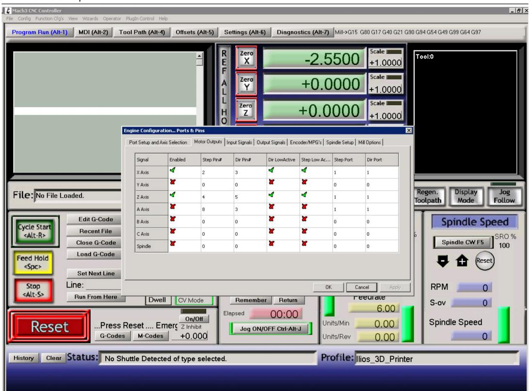
If you purchased the High Torque setup, set the signals and pins as shown on the image above.
