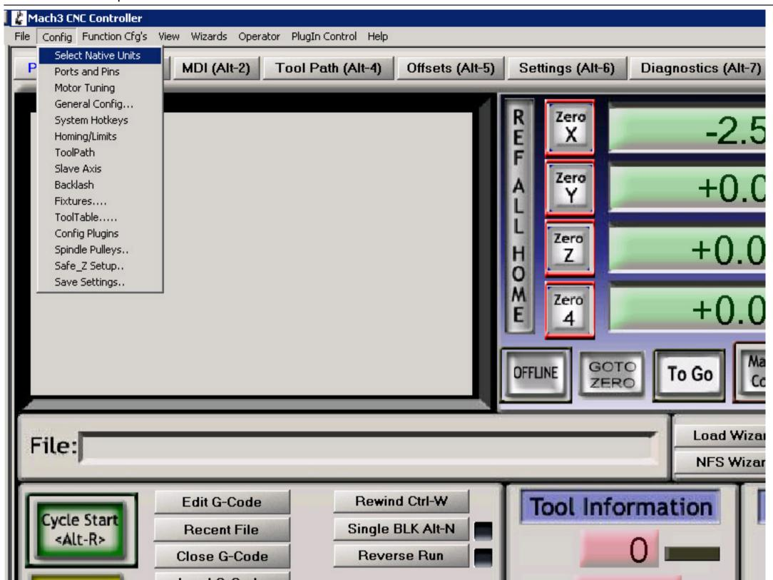
The first thing we need to setup are the units we shall be using. Please note that although many countries use different units, the Ilios Kit and all instructions for it as well as the script which runs the machine is in Metric units.
