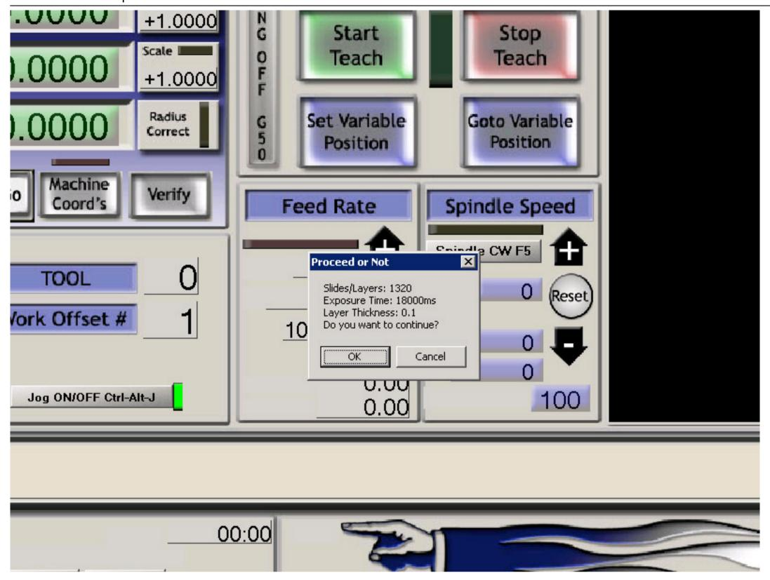
Before the script begins its task, it shall ask you if the parameters that are set are correct. For the time being the parameters of the script like the Layer Thickness, Power Point folder, Number of layers and exposure time are set manually by simply opening the script with a Text editor.
