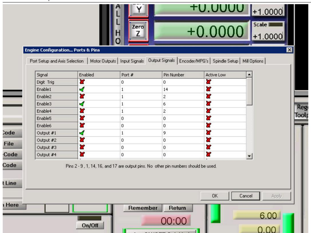
Besides the motor control, there are also additional signals which enable each motor and other hardware. In the Output Signals tab set everything up as shown. Although we are not using the Y axis, it is still a good idea to enable it for later use. As far as signals go, this is the only setup you need to do.
