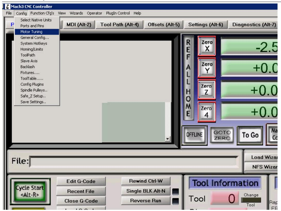
In the next step, we tell Mach the motor specifications and set some boundaries for the acceleration and motion of each axis. Use the Motor Tuning tab to set this up.
