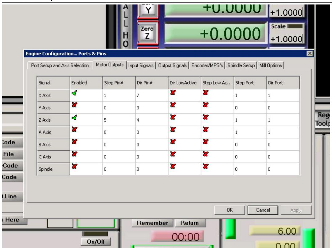
We now need to setup the actual signals that are going to be controlling our motors. Since both Z axis motors, as described in the Electronics Setup are connected together, we only need to setup two axises. Configure the signals and the Direction of your setup as shown on the image above.
