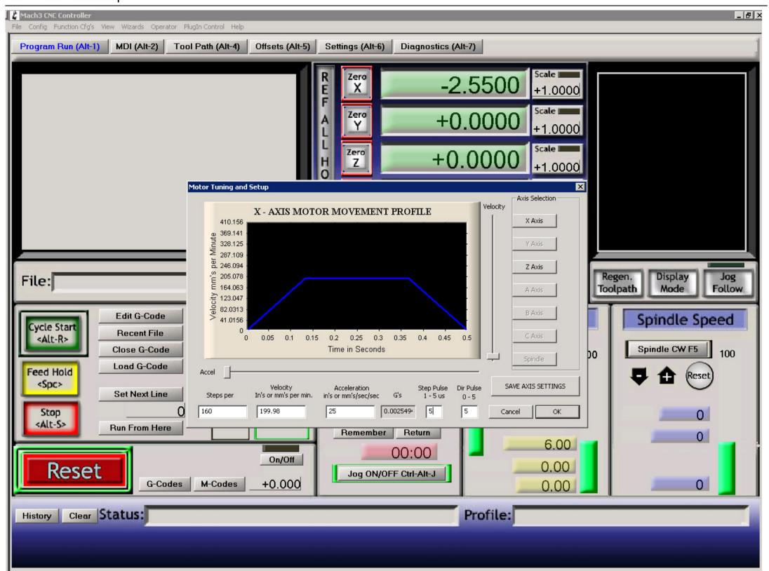
Note that for the High Torque setup, the "Steps per" parameter should be <u>160</u> and NOT 80 as with the default setup. High Torque motors do twice as many steps for the same distance, thus provide higher resolution by default.
