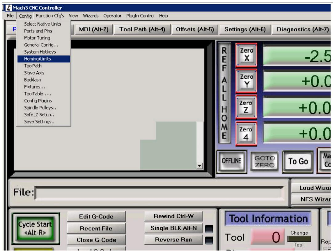
One last setup before we can use Ilios. We need to set some boundaries for the machine, so it knows where to stop and where to go to Home the platform. Use the Homing/Limits tab to set this up.
