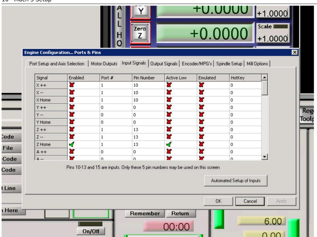
If you purchased the <u>Complete Ilios HD Kit</u>, you should have only one sensor, which determines the Home position of the machine. Set the signals as shown above to enable this sensor.
