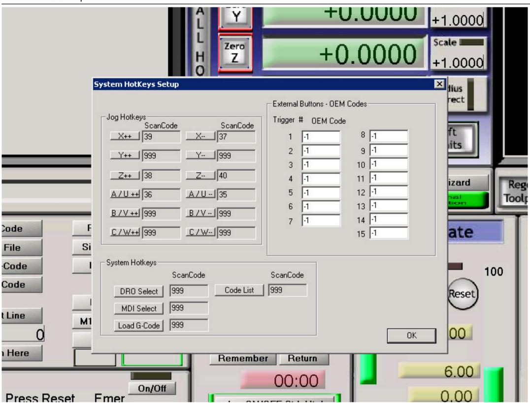
This is quite simple. We need to control only the Z+ and Z- as well as X+ and X- movements. Press the button on the screen for each motion and then press the key on your keyboard to acknowledge your selection. Normally these movements are set to the Up/Down and Left/Right arrow keys on your keyboard. Press OK to save your setup.
