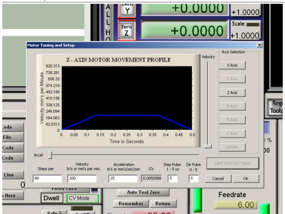
Use the same settings for the Z axis as you did for the X. The motors and all the hardware is the same. Don't forget to Save the Axis before exiting.
